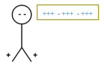
Polarized by a positive object. It is polarized because the charges are separated. We know that the object that polarized it is positive because electrons are attracted to the top and away from the bottom
