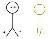
This is a neutral electroscope. Positives and negatives are balanced.
