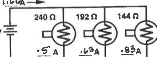
$$P = 60 \text{ W} \quad P = 75 \text{ W} \quad P = 100 \text{ W}$$
