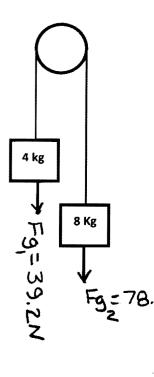
Solve for the acceleration using Newton's Second Law. Consider the whole system as a single mass.
