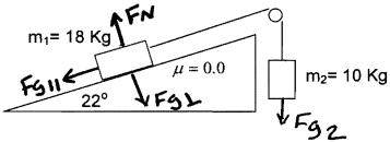
Calculate the acceleration and force of tension of the system.
