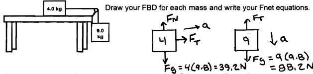
Calculate the force of tension and the acceleration of the system if  $\mu = 0.0$
